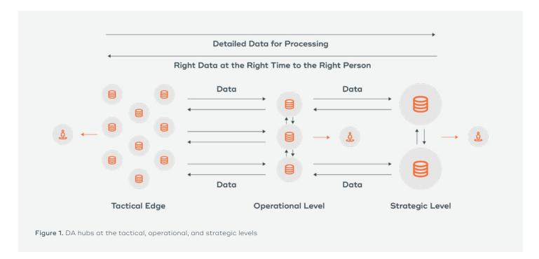
Each circle in Figure 1 represents DA hubs distributing data to other DA hubs, different combat systems, or personnel. DA hubs exist on three levels: the tactical edge, the operational level, and the strategic level. Data flows from the tactical edge to the strategic level to support broader data analysis and analytic modeling. Likewise, data that flows down to the tactical edge is available to personnel in the field.
